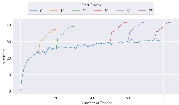
Figure 4: Applying our strategy to improve performance. The blue curve corresponds to the accuracy of the original CLIP model. Each other curve represents the zero-shot accuracy of the CLIP model after applying our strategy with different starting points. For example, the orange curve corresponds to applying our strategy on the CLIP model after it has been trained for 10 epochs (out of 75 epochs in total). Note that applying our strategy earlier during training leads to a performance improvement beyond the final accuracy reached by the model trained for 75 epochs. See Appendix B for additional results.
