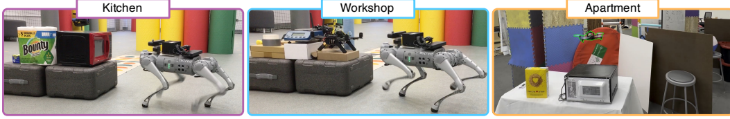
Figure 4: Stillshots of a quadruped mapping different areas of a kitchen and workshop and a drone mapping an apartment-like scene. Each robot trains independent GSplat submaps of the areas it mapped. The submaps of each scene are registered to obtain a composite map covering the entirety of the scene.
