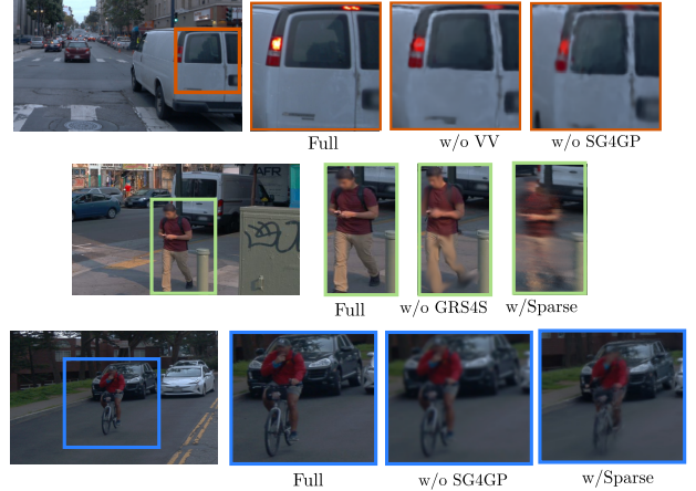
Figure 5. Ablation Analysis Our ablation analysis confirms the need for dense representations of thin objects like pedestrians and cyclists (rows 2 and 3). Furthermore, removing SDF guidance for Gaussian primitive distribution adversely impacts rendering quality (rows 1 and 3).
