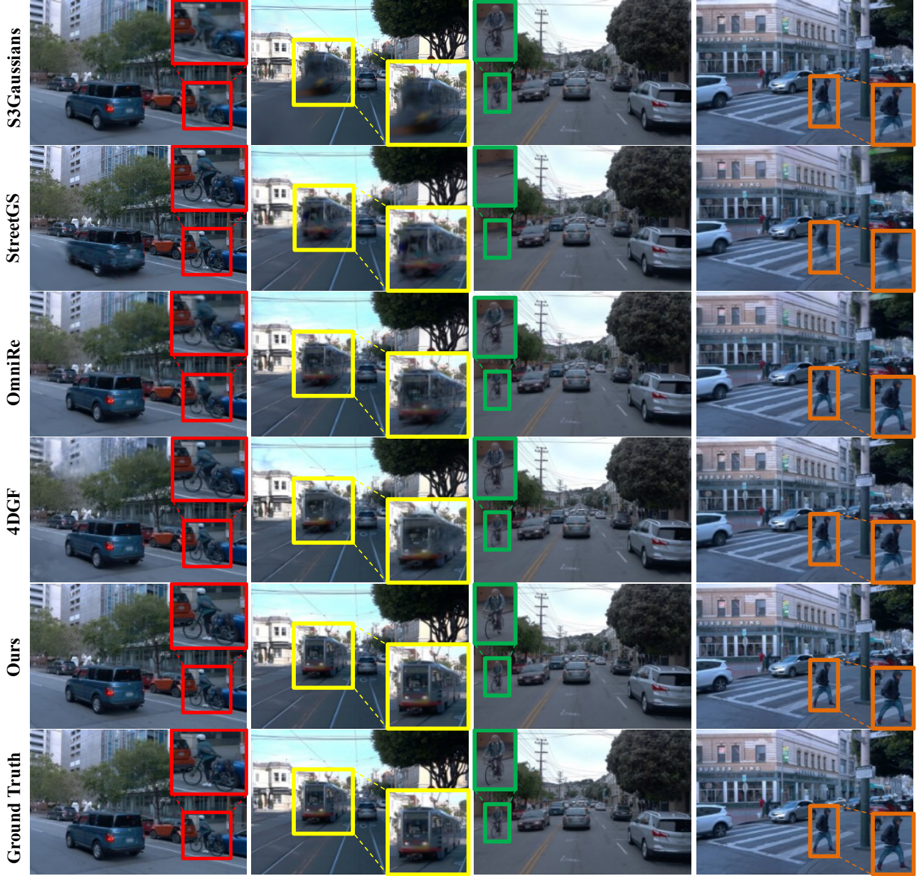
Figure 6. Qualitative comparison of baselines and our method on the NOTR Dataset with zoomed in regions We show results on some atypical objects observed in urban scenes namely: a tram and two cyclists, as well as a pedestrian. Some of these are tricky cases not always very well modeled by some or all of the baselines. In contrast UGSDF achieves a very high level of fidelity in novel view synthesis for these objects.
