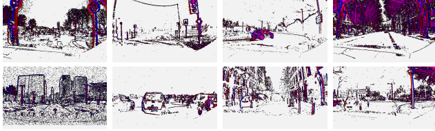
Figure 2. Event-based Camera Output Visualization. Sample frames from the 1Mpx dataset showing event polarity. Red indicates positive events, and blue denotes negative events.
