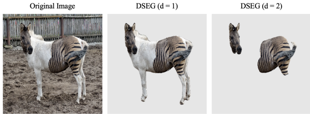
Figure 11: Misclassification example. The image depicts a hybrid of a horse and zebra that EfficientNetB4 classifies as a zebra with p = 0.17 . DSEG-LIME, with a depth of one, highlights the entire animal, offering a broad explanation. Meanwhile, DSEG at depth two pinpoints specific zebra-like patterns that influence the model’s prediction. This suggests that the model is fixating on particular visual features associated with zebras, explaining its erroneous classification.
