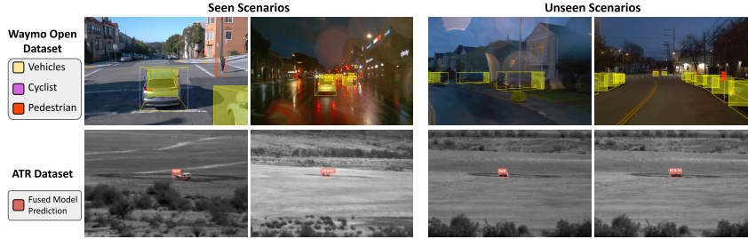
Figure 4: Qualitative examples of VLC Fusion in both seen and unseen environments. Top row: 3D detections on the Waymo Open Dataset under seen and unseen conditions, with vehicles (yellow), cyclists (purple) and pedestrians (red) accurately localized. Bottom row: 2D detection on the ATR dataset for seen and unseen scenarios. More qualitative examples are provided in App. G.
