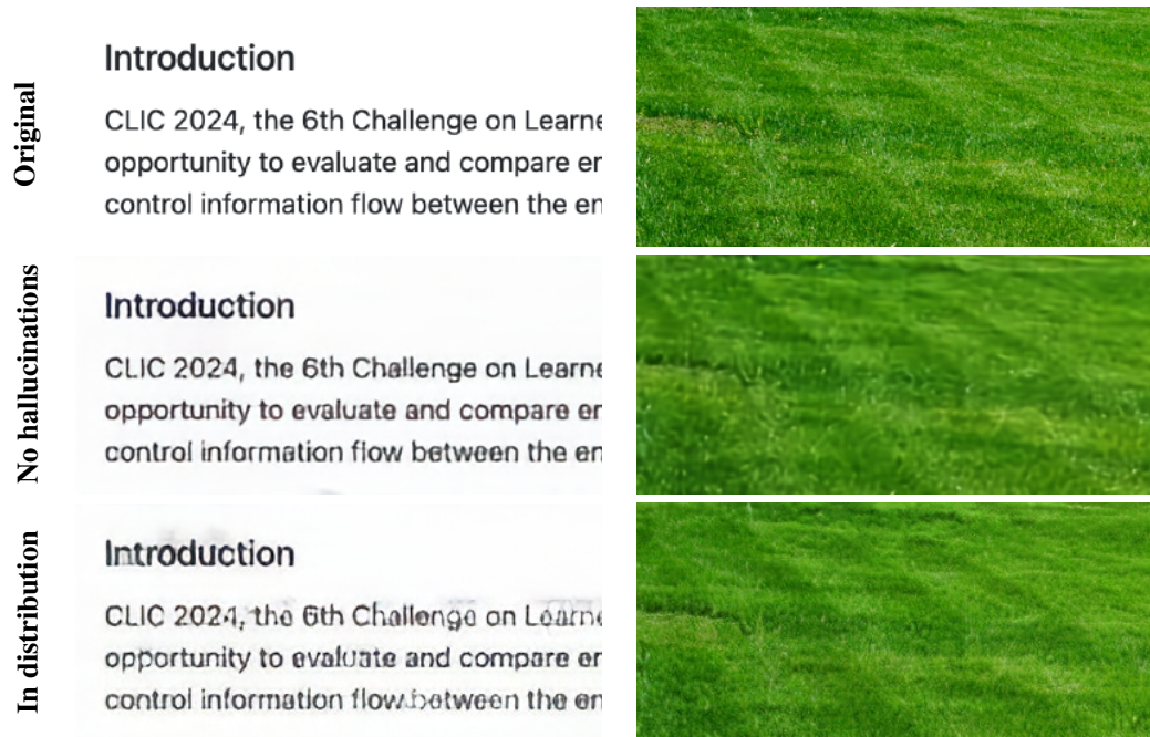
Figure 1: 1) Original image 2) compressed with an MSE distortion optimized model 3) compressed with a hallucinating MSE+GAN optimized model. For the left image containing text, hallucinations degrade the image quality. For the right image containing grass, an in-distribution sample with hallucinations produces a higher perceptual quality.
