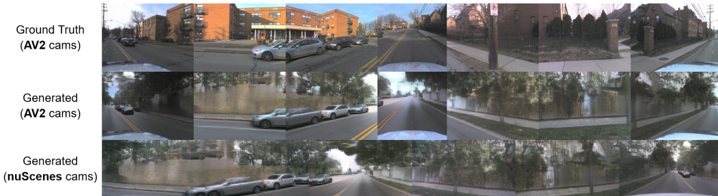
Figure 1: Autonomous driving scene synthesis from AV2 to nuScenes. BEV-VAE with DiT generates a BEV representation from 3D bounding boxes of AV2, which can then be decoded into multi-view images according to the camera configurations of nuScenes.
