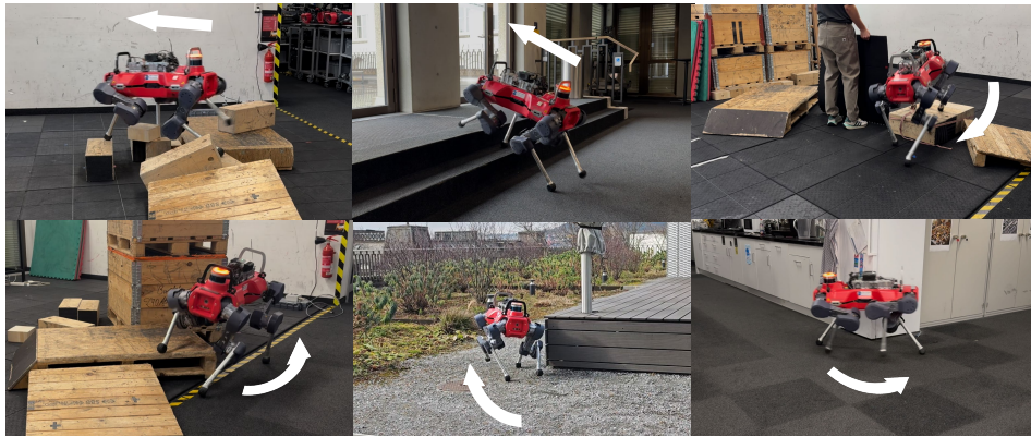
Figure 1: ANYmal-D hardware experiments in indoor/outdoor terrains (stairs, random blocks, high obstacles). The white arrow marks the direction of movement toward the specified goal position. The robot employs an animal-like gait to traverse uneven ground and avoid obstacles, demonstrating our policy’s transfer of flat-ground motion priors to complex environments. (See supplementary videos at https://anymalprior.github.io/ )
