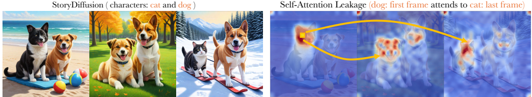
(b) Visualizing self-attention leakage . We find that intercharacter leakage (a) occurs due to exacerbated self-attention leakage where tokens from one subject ( dog ) pay attention to tokens from another subject ( cat ).
