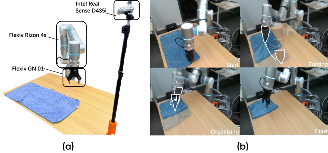
Figure 9: Real World Experiments. (a) The hardware platform setup used for data collection and policy evaluation. (b) A representative execution sequence of the towel folding task.
