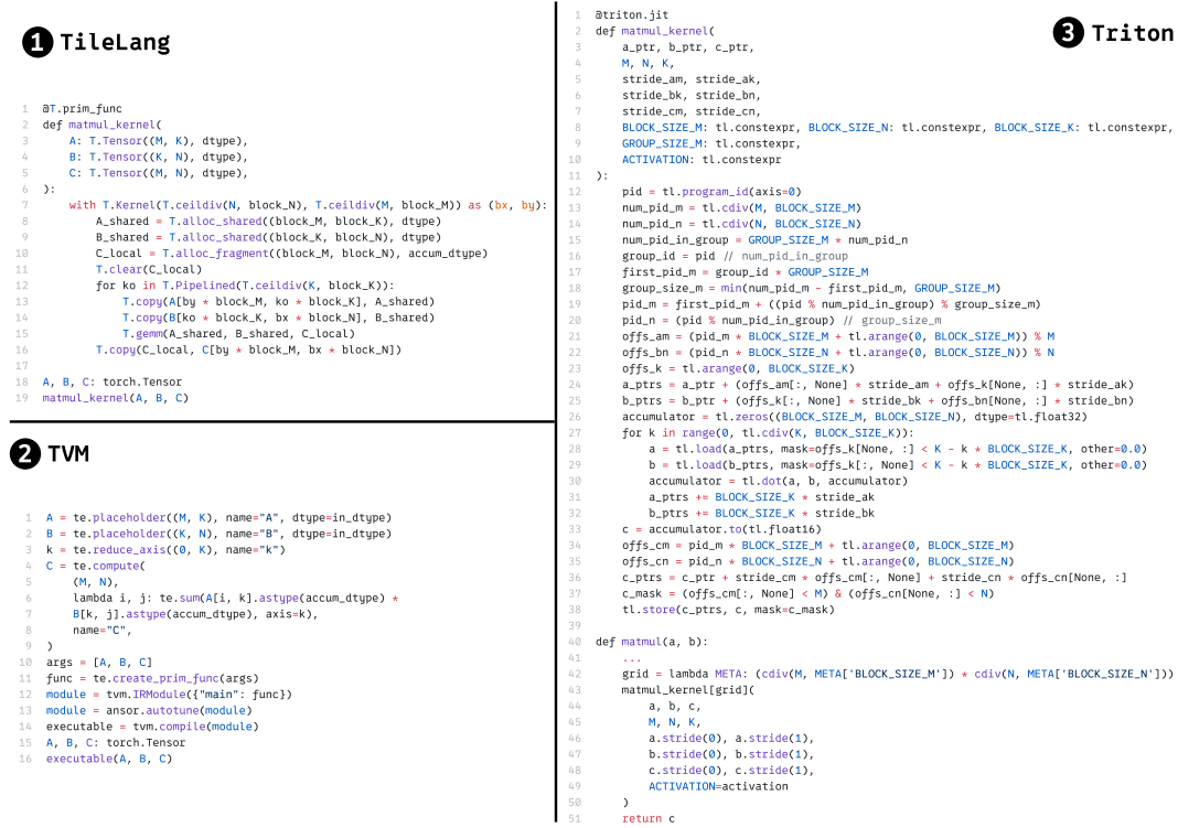
Figure 12: Side-by-side diff of minimal GEMM implementations in TVM, TILELANG, and Triton (first page).
