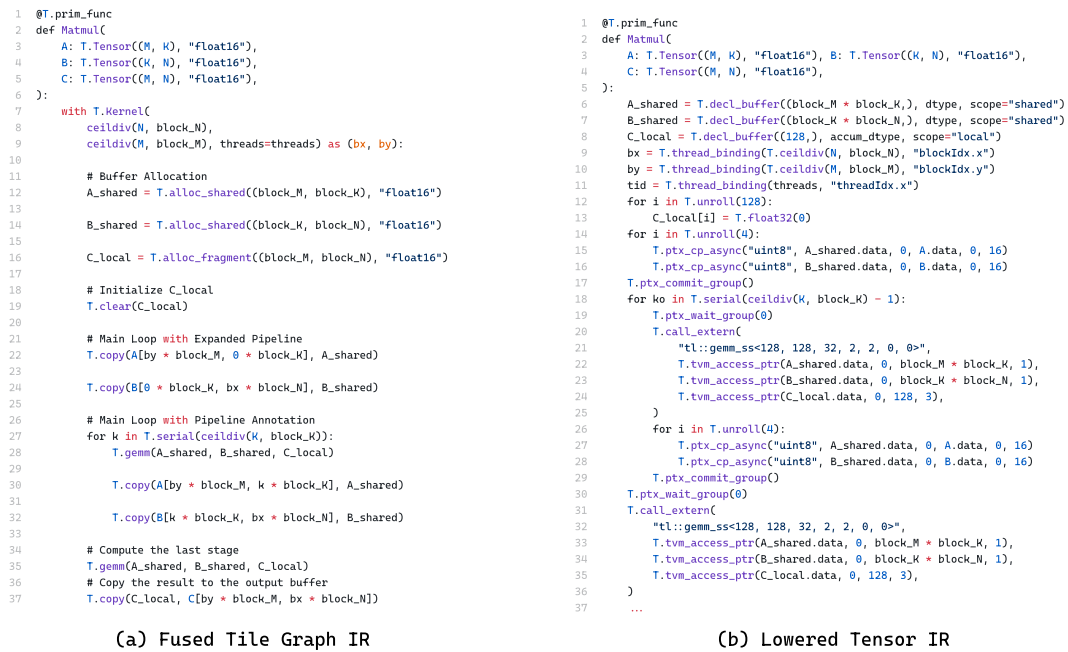
Figure 13: A side-by-side comparison showing how tile-level FTG-IR is lowered into Tensor IR.
