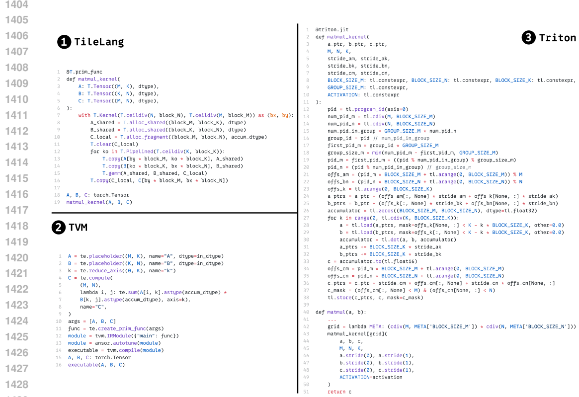
Figure 12: Side-by-side diff of minimal GEMM implementations in TVM, TILELANG, and Triton (first page).
