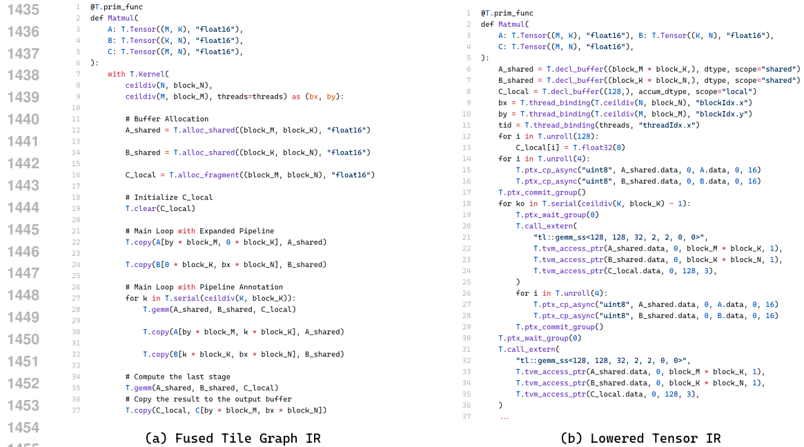
Figure 13: A side-by-side comparison showing how tile-level FTG-IR is lowered into Tensor IR.
