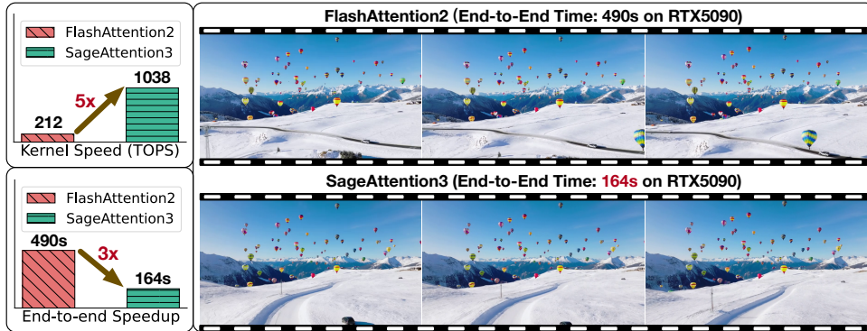
Figure 1: The upper left figure shows the kernel speedup on RTX5090. The other two figures show the end-to-end inference speedup of generating a video using HunyuanVideo on RTX5090. Note that FlashAttention3 can only run on Hopper GPUs, so FlashAttention2 is already the fastest on RTX5090.
