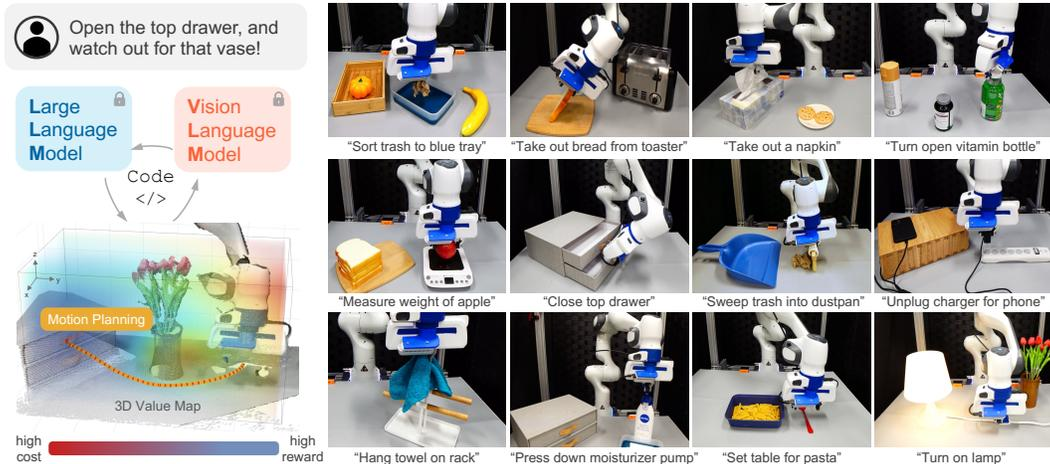
**Figure 1: VOXPOSER** extracts language-conditioned **affordances** and **constraints** from LLMs and grounds them to the perceptual space using VLMs, using a code interface and without any additional training. The composed map is referred to as a 3D value map, which enables **zero-shot** synthesis of trajectories for large varieties of everyday manipulation tasks with an **open-set of instructions** and an **open-set of objects**.
