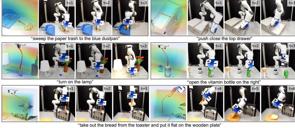
**Figure 3:** Visualization of composed 3D value maps and rollouts in real-world environments. The top row demonstrates where “entity of interest” is an object or part, and the value maps guide them toward target positions. The bottom two rows showcase tasks where “entity of interest” is the robot end-effector. The bottom-most task involves two phases, which are also orchestrated by LLMs.
