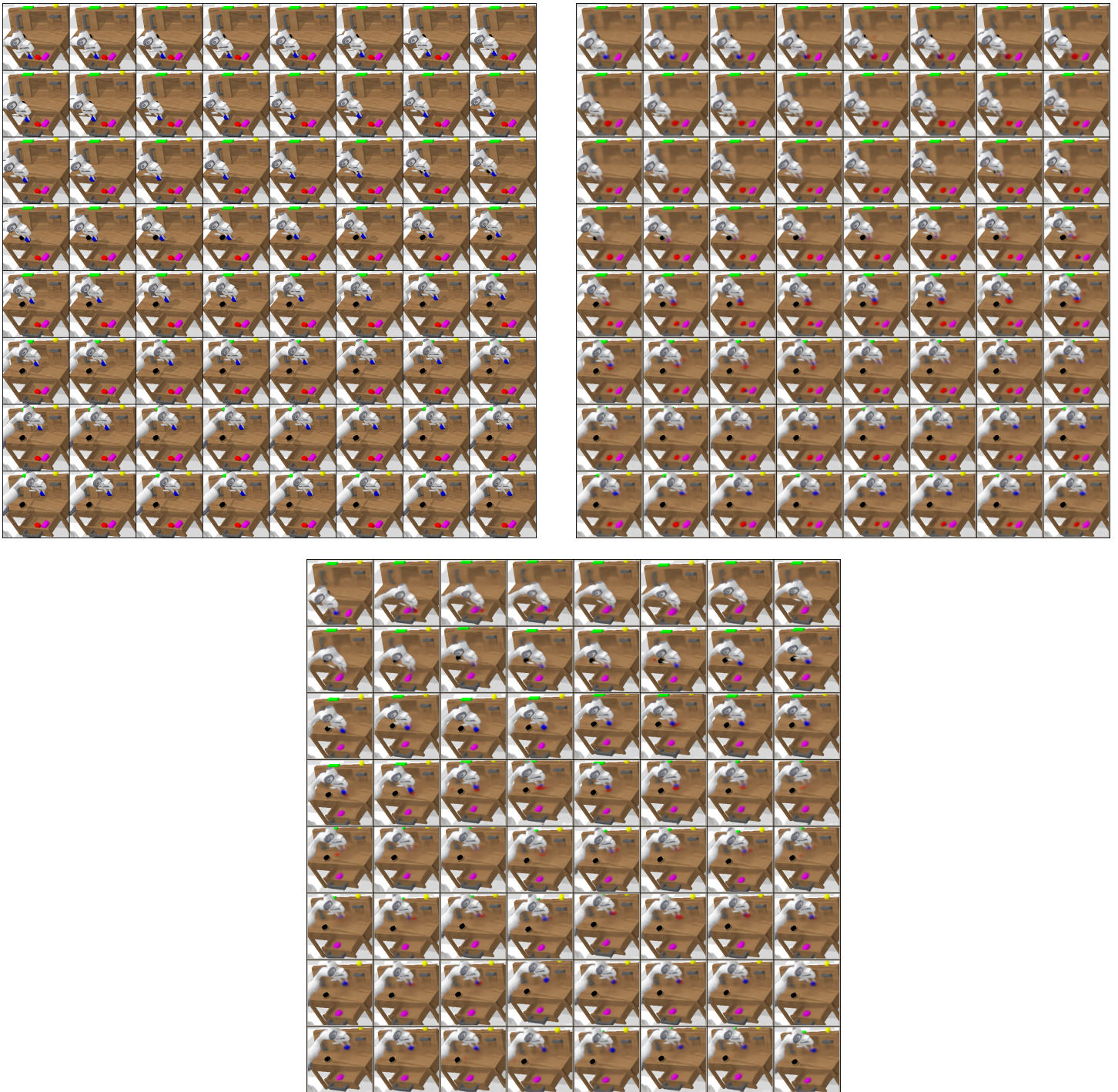
Figure 4: Comparison of a ground truth trajectory for the "place in slider" task (left), the reconstructed trajectory (right), and the generated trajectory through denoising (bottom).
