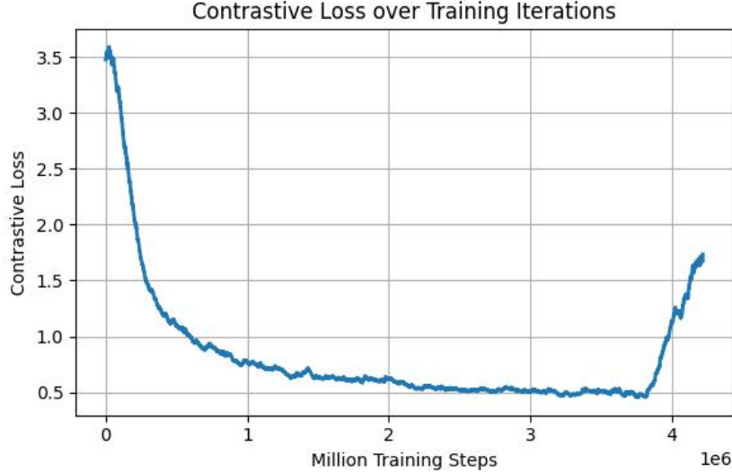
Figure 12: Contrastive loss tracked over the course of the training. After 3.8 million steps, the loss increases again, causing the training to collapse.
