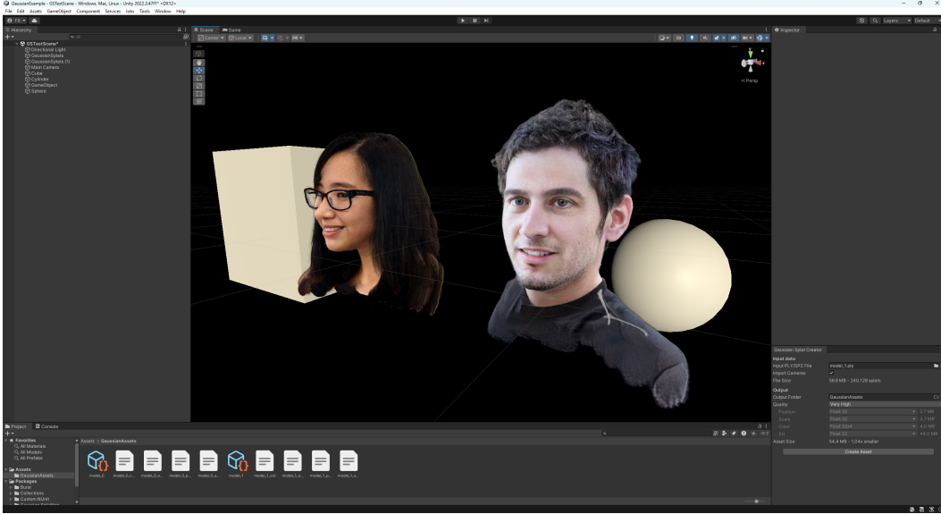
Figure 15: Our faces imported into unity using the Unity Gaussian splatting plugin by Aras Pranckevičius: https://github.com/aras-p/UnityGaussianSplatting
