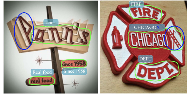
Fig. 9. Failure cases. Green polygons represent predicted detection results, and blue circle represents error detection regions. The dashed boxes stand for predicted recognition results, and blue characters are error recognition results.
