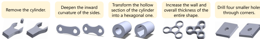
Figure 1: Text-based CAD Editing achieved by CAD-Editor. Each sub-figure shows the textual instruction at the top, the original CAD model on the left, and the edited CAD model on the right. The rendered image is shown for better comprehension. The actual editing occurs on sketch-and-extrusion (SE) operations of a CAD model to provide editability and reusability.
