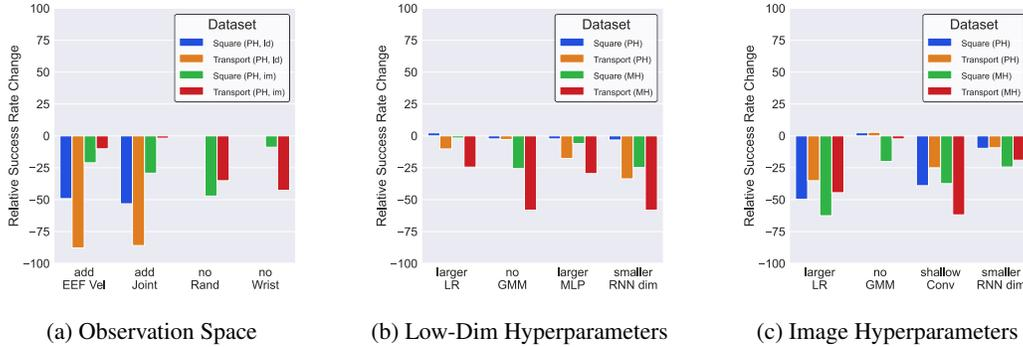
Figure 2: **Effect of Observation Space and Hyperparameter Choice.** We show how the success rate that BC-RNN obtains can drop drastically due to changes to the observation space and hyperparameter settings.
