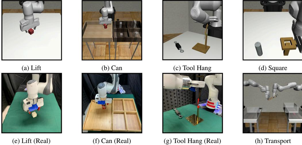
Figure 1: **Tasks.** We collect datasets across 6 operators of varying proficiency and evaluate offline policy learning methods on 8 challenging manipulation tasks that test a wide range of manipulation capabilities including pick-and-place, multi-arm coordination, and high-precision insertion and assembly.
