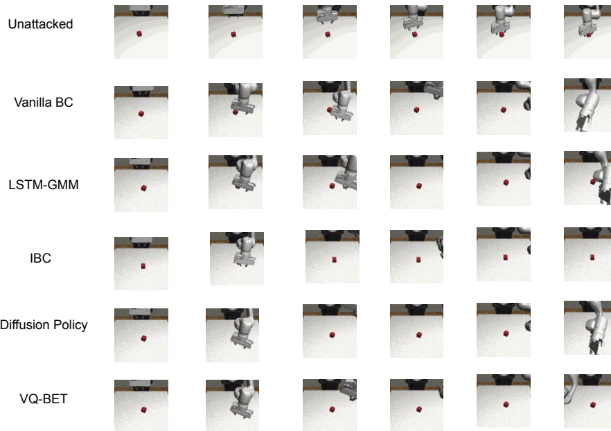
Figure 8: Targeted Attacks on Lift task, where the target direction is towards top-left corner of the object.
