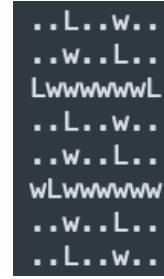
Figure 7: Minigrid floorplan that we used for generating problem instances. L represents locked doors, w represents blocked places which can't be crossed, and all other dots represent places where the agent can walk. In each problem instance, the robot start and end location are chosen randomly. The keys are spread around the map, not depicted in this figure.
