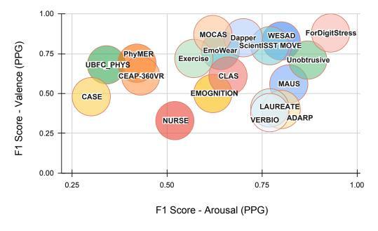
Figure 12: **Benchmarking results: PPG only.** This bubble plot illustrates the impact of PPG signals on F1 performance (best model) for arousal and valence classification across 19 datasets.
