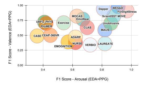
Figure 13: **Benchmarking results: EDA + PPG combined.** This bubble plot illustrates the impact of combining EDA and PPG signals on F1 performance (best model) for arousal and valence classification across 19 datasets.
