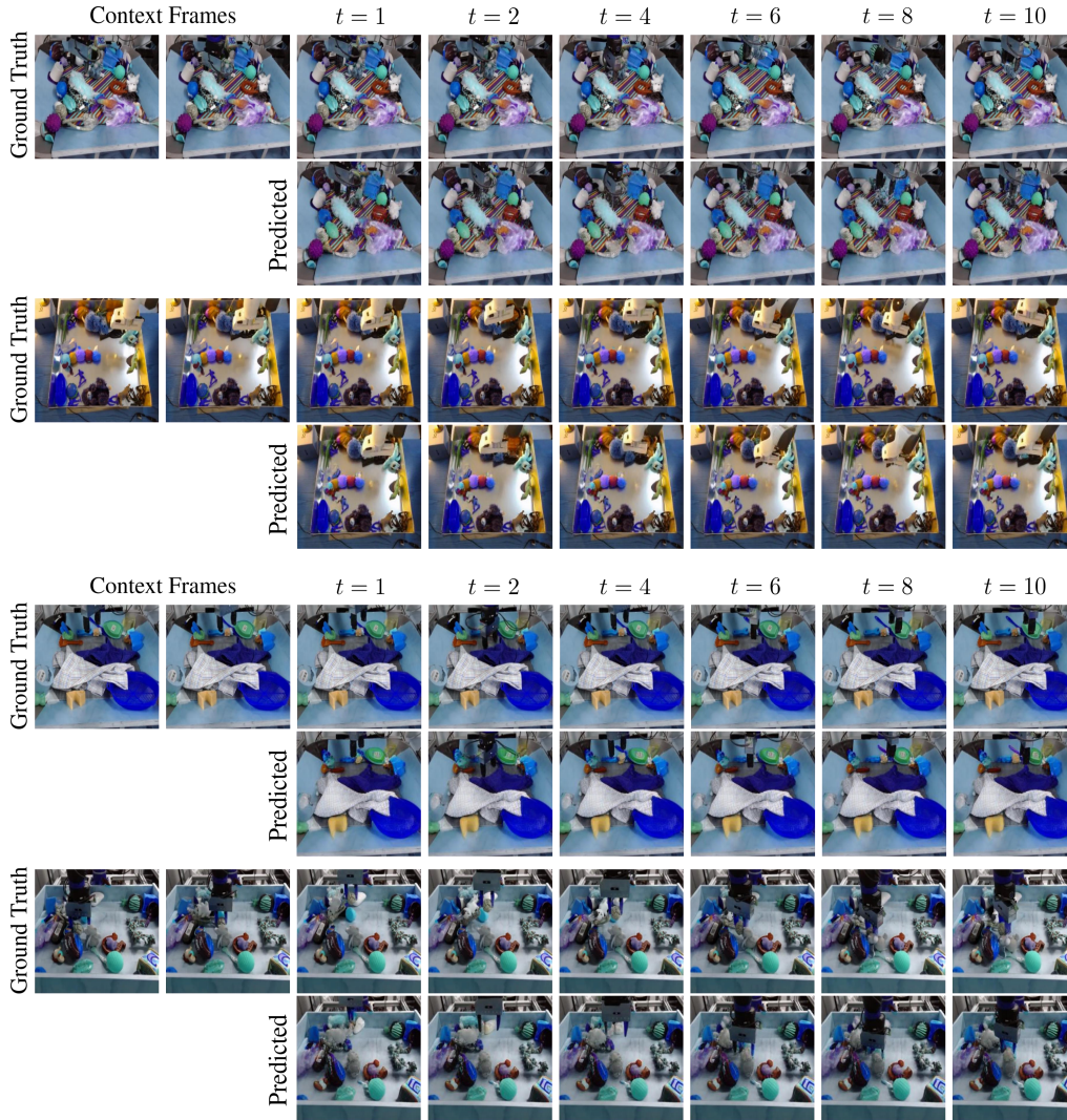
Figure 11: 256 \times 256 future frames predicted by HARP on RoboNet dataset.
