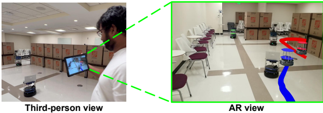
Figure 4: Mock warehouse and AR visualizations that include robot avatars and trajectories in color.
