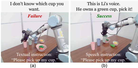
Figure 1: For personalization tasks, (a) previous VLAs with text instructions fail, while (b) our VLAS with speech instructions could successfully address them.
