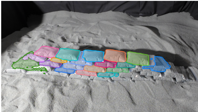
Fig. 3: Visual segmentation of individual sandbags while stacked on the structure. Texture blend can lead to incorrect segmentation, as shown on the bottom left side of the structure.
