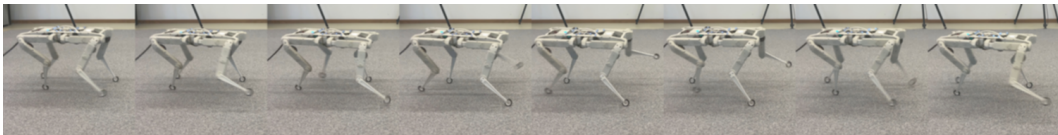
(c) Trot locomotion with high base height.
