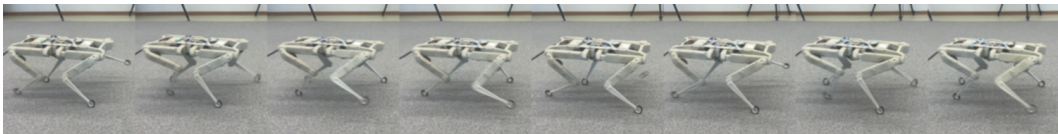
(b) Trot locomotion with middle base height.
