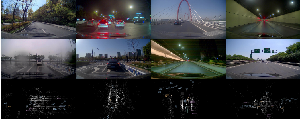
Figure 1: Images and point clouds sampled from the ONCE (One million sCenEs) dataset. Our ONCE dataset covers a variety of geographical locations, time periods and weather conditions.
