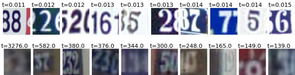
Figure 5: The data with the lowest (top) and highest (bottom) predicted temperatures in the SVHN dataset. High temperature entries are blurry, cropped poorly, and generally difficult to classify.
