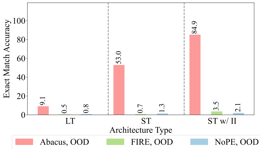
Figure 14. Effect of removing the masking of the loss before the “=” sign in the addition task. All models perform worse when trained for 24 hours on a single Nvidia RTX4000 if we do not mask the input question in the loss function.
