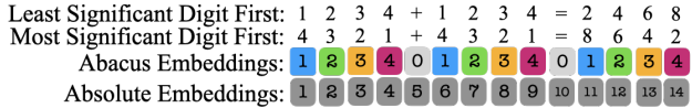
Figure 1. Visualization of data formats and positional embeddings. Abacus Embeddings give the same positional embeddings to all digits of the same significance.
