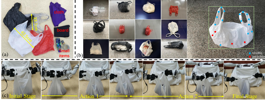
Figure 2: (a) Plastic bags and fillers used in this work. We give demonstrations on white, red and black bags. The grey plastic bag is used to show the generalization of IIM. We fill plastic bags with different items varying in size and shape, including cloths, paperboards, bottles, tape volumes, and dry batteries. (b) The PBPose dataset. Images are captured in various backgrounds, knotting states, occupied states, illumination conditions, placement status (standing or lying down), and angles of view. (c) We design two motion primitives for tying an Ian Knot in the air.
