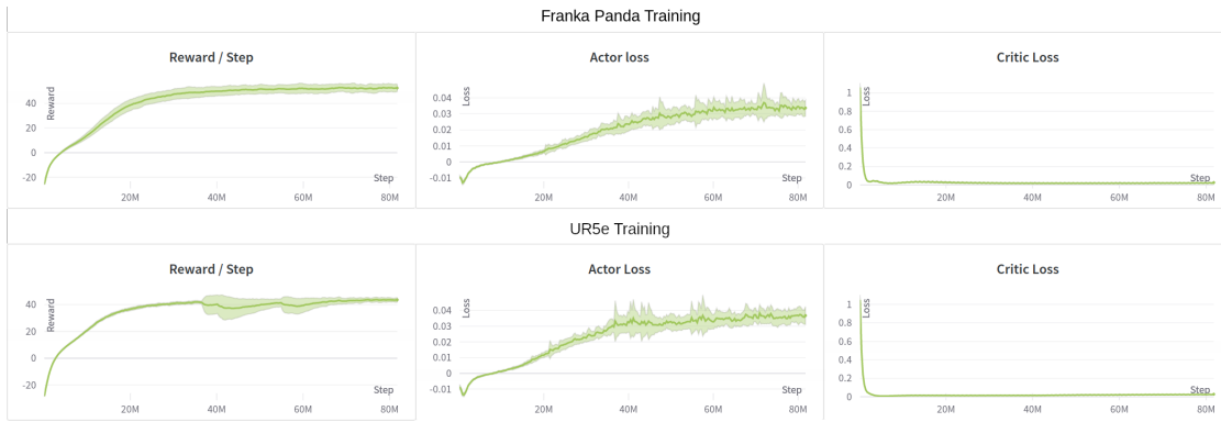
Figure 6. Low-level training graphs. The task is solved upon reaching a mean reward of 40. UR5e achieves a better score due to a reduced workspace and a lower number of joints to be controlled.
