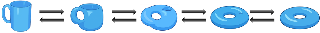
Figure 2: Topological Equivalence : Both a coffee cup and a donut have one hole and can be mutually transformed via continuous deformation without tearing or gluing. They are regarded as topologically equivalent.
