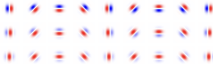
Figure 10: Rotating Gabor functions: \mathbf{f}_1(x) = \sin(x) , \mathbf{f}_2(x) = \sin(x + \frac{\pi}{4}) , \mathbf{f}_3(x) = \sin(x + \frac{\pi}{2}) . The plots demonstrate how the Gabor filters rotate with respect to phase shifts.
