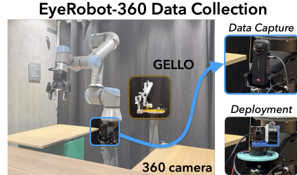
Figure 5: Teleop Data Setup with EyeRobot . We collect actions with GELLO [64], and the EyeGym environment with a time-synced 360 camera.
