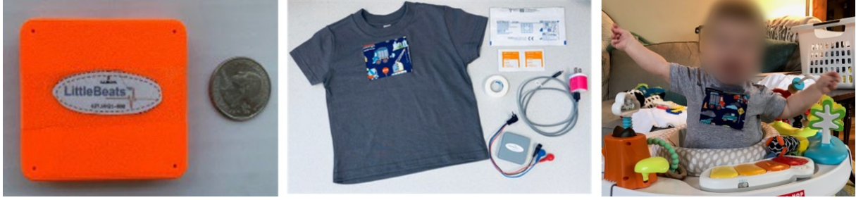
Figure 3: (A) LittleBeats device case; (B) LittleBeats supplies, including electrocardiogram leads, electrodes, charger, and shirt; and (C) an infant wearing LittleBeats at home.
