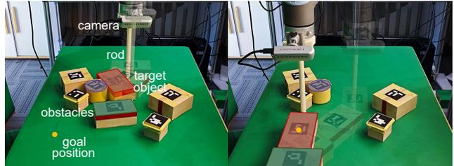
Fig. 1. Object retrieval task through planar pushing. The target object in red is separated from the clutter with a rod-like pusher through pushing manipulation. **Left:** The purple cylinder is pushed aside and the target object quickly navigates through fixed obstacles on both sides. **Right:** the cyan cube is pushed away and the target object bursts through the clutter.
