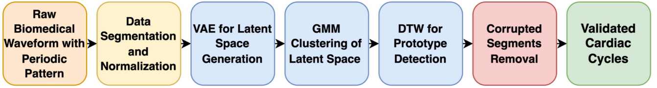
Fig. 1. Variational Autoencoder-based framework for periodic biomedical signal validation.
