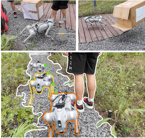
Figure 5: Robot obstacle avoidance performance was assessed in varied scenarios, including complex terrain and dynamic human interference.
