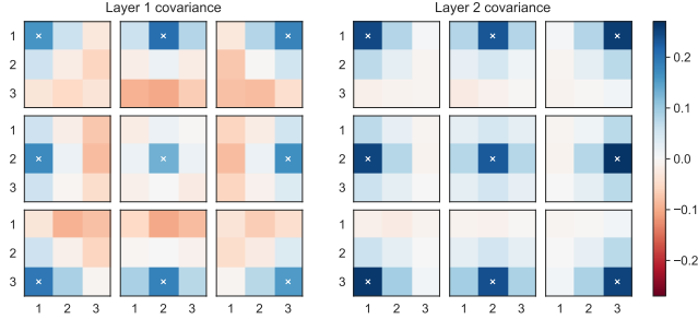
Figure 3: Spatial covariance of the weights within CNN filters, multiplied by the number of input channels (1 for Layer 1, 64 for Layer 2). The weights correlate strongly with neighboring pixels, and anti-correlate (Layer 1) or do not correlate (Layer 2) with distant ones. Each delineated square shows the covariances of a filter location (marked with \times ) with all other locations.
