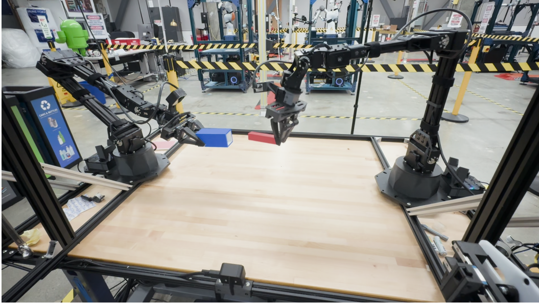
Figure 12: Real-world replica of our simulated Aloha Single-Insertion task
