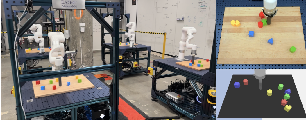
Figure 6: LanguageTable Environments. Left The four LanguageTable robot stations used for our real-world experiments. Right, Top Camera view of the real-world LanguageTable robot station. Right, Bottom Camera view of the simulated LanguageTable robot station.
