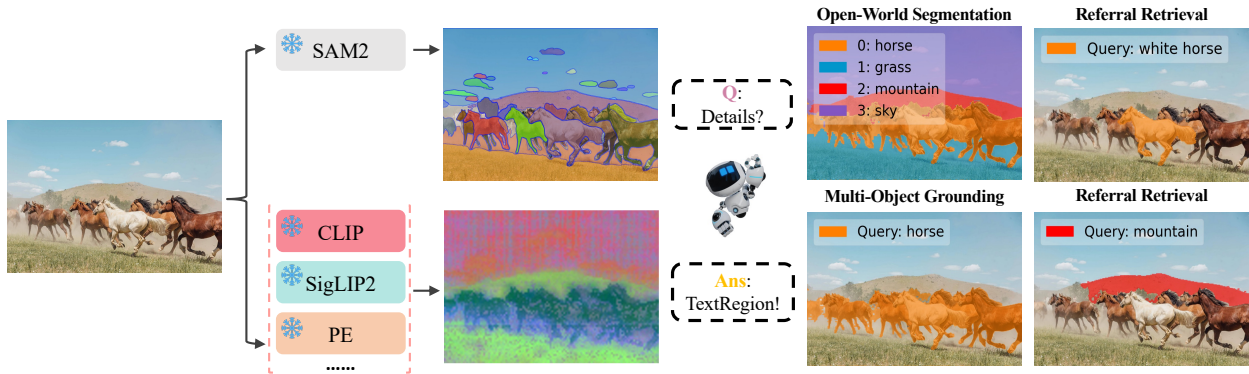
Figure 1: Using feature maps from frozen image-text models and segment masks from SAM2, we generate text-aligned region tokens that can be directly applied to various downstream tasks.
