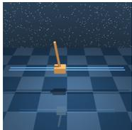
Figure 19: **Cartpole(4, 1, 5)**: This domain features a cart connected to a pole via an unactuated joint. It encompasses a set of four distinct tasks. In the context of our experimental setup, we focus on the `swingup` task. Here, the pole is initially positioned downward, and the objective is to apply appropriate forces to the cart to swing the pole upward and maintain its upright position.
