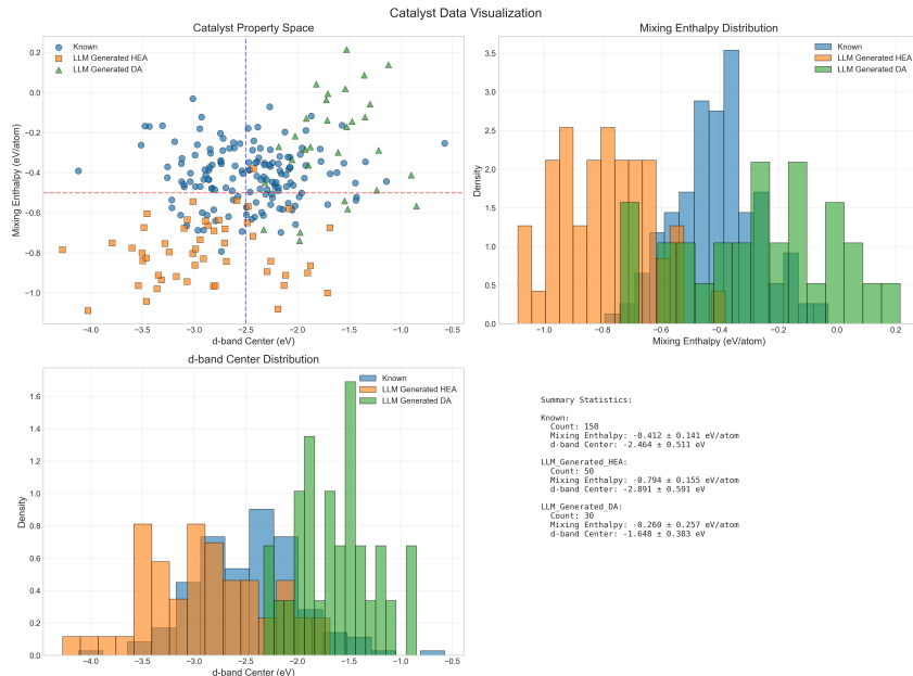
Figure 2: Comprehensive comparison of material properties between known catalysts and LLM-generated catalysts (HEA: High-Entropy Alloy, DA: Doped Alloy). The visualization maps catalysts by mixing enthalpy and d-band center, with LLM-HEAs occupying the favorable lower-left quadrant. Property distributions show LLM-HEAs exhibit more negative mixing enthalpies (mean -0.794 eV/atom) indicating higher stability, and more negative d-band centers (mean -2.891 eV) correlating with enhanced catalytic activity.
