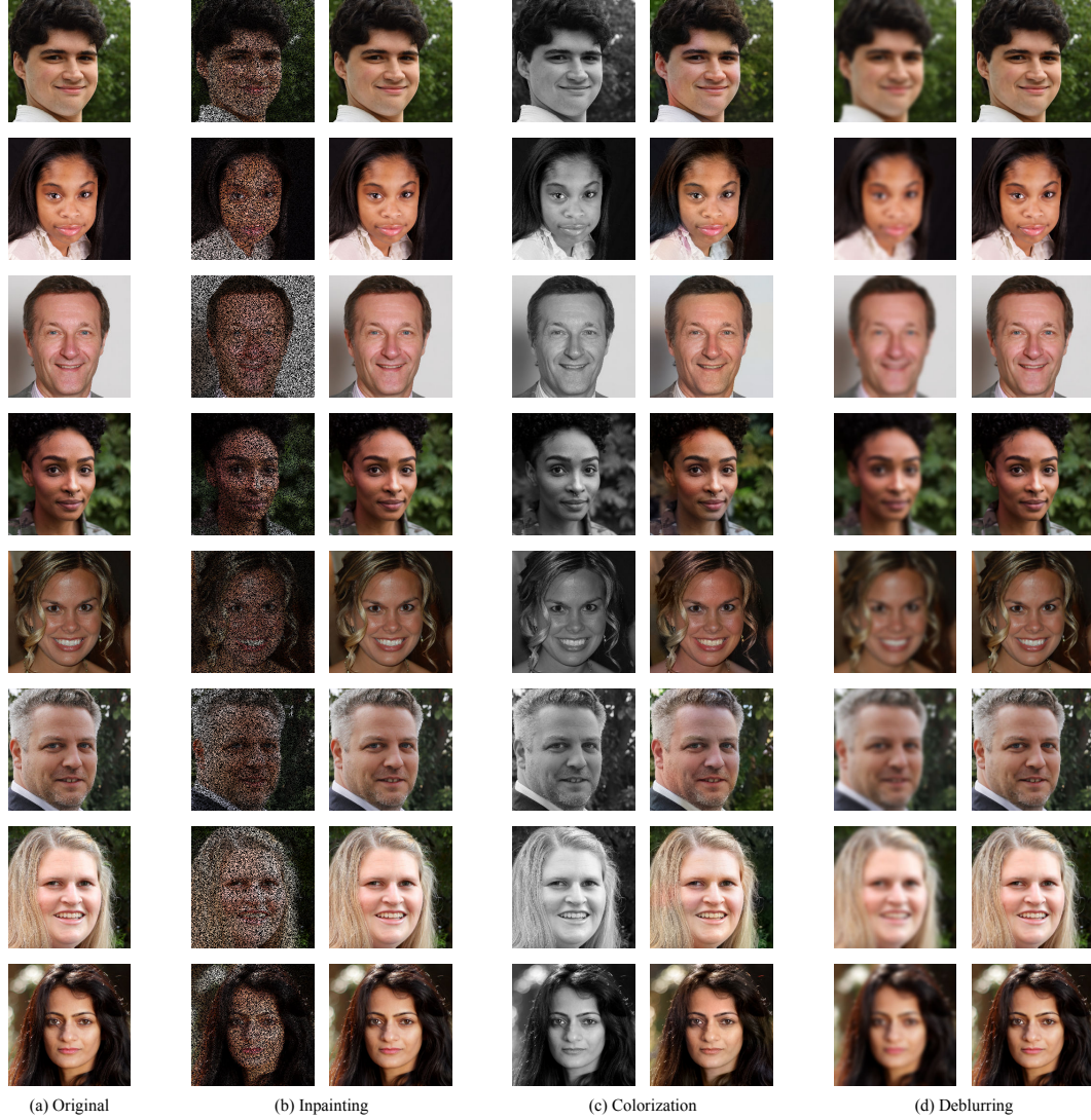
Figure 18: Image inpainting, colorization, and deblurring results of RDIM-10 on images from the FFHQ dataset. For inpainting, pixels in the original images are randomly masked and set to zero with probability p_{\text{mask}} = 0.5 . For colorization, grayscale inputs are obtained by converting the original RGB images to luminance. For deblurring, synthetic blurred images are generated from ground truth images by applying a Gaussian blur with kernel size 15 \times 15 and standard deviation \sigma = 3.0 . RDIM is trained with T = 50 and \gamma = 3.0 . Inference is conducted with S = 10 and \eta = 1.0 . In (b), (c) and (d), the left side represents the input image and the right side the output.
