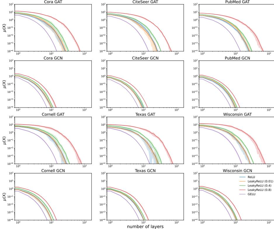
Figure 1: Evolution of  $\mu(X^{(t)})$  (in log-log scale) on the largest connected component of each dataset (top 2 rows: homophilic graphs; bottom 2 rows: heterophilic graphs). Oversmoothing happens exponentially in both GCNs and GATs with the rates varying depending on the choice of activation function. Notably, GCNs demonstrate faster rates of oversmoothing compared to GATs.
