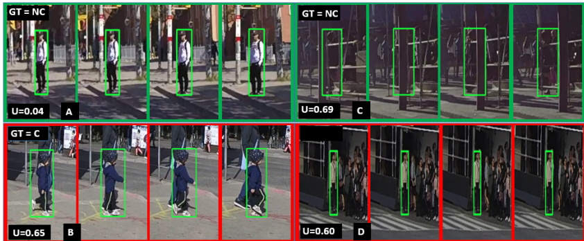
Figure 7: Examples for low (A) and high uncertainty (B), (C), (D) samples from PIE dataset. GT: Ground Truth (C/NC) and epistemic uncertainty (U) are marked on top and bottom of the snippets respectively. Snippets encapsulated in red indicates wrong model prediction and green encapsulation indicates correct model prediction.
