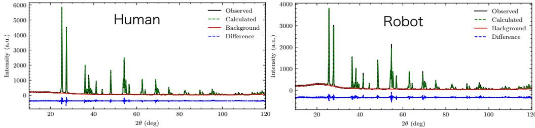
Figure 5: Comparison of the XRD patterns and Rietveld refinement results for samples prepared by manual operation and the robotic arm (80 mg).
