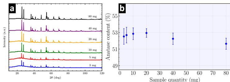
Figure 6: XRD analysis of TiO<sub>2</sub> samples with varying quantities. (a) XRD patterns for different sample quantities. (b) Effect of sample quantity on anatase content precision, with error bars representing standard deviation.
