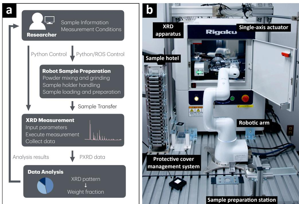
Figure 1: Autonomous PXRD system overview. (a) Schematic of the autonomous PXRD experimental workflow. (b) Key components of the system setup.
