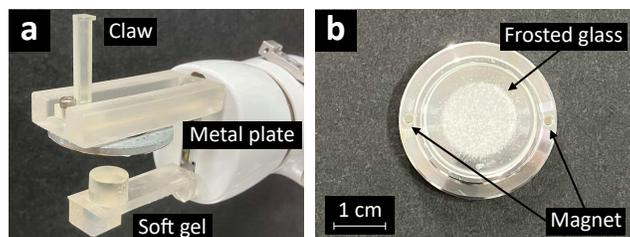
Figure 2: Close-up view of the key components of the autonomous PXRD system. (a) Multifunctional end effector. (b) Custom-designed sample holder.
