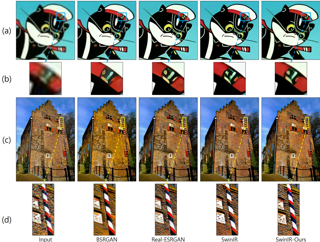
Figure 5: Illustrative example highlighting color distortion and texture smearing. In the second row of Real-ESRGAN (Wang et al., 2021; 2018b) results, the circle on the right, initially red, has undergone a distortion leading to a yellow coloration. Similarly, in the third row with BSRGAN (Zhang et al., 2021) results, a discernible shift in the overall building color is evident. Moving to the fourth row featuring SwinIR, the texture of the surrounding brickwork has blended into the striped pattern of the chimney. We used SwinIR (Liang et al., 2021) as our SR backbone in here. Best viewed in zoom.
