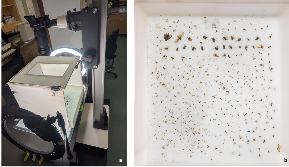
Figure 4: (a) Imaging setup used to capture bulk images of the MassID45 dataset, including the positioning of the camera, light cube and ring light sources. (b) A representative image captured using the described imaging setup, with the sides trimmed.
